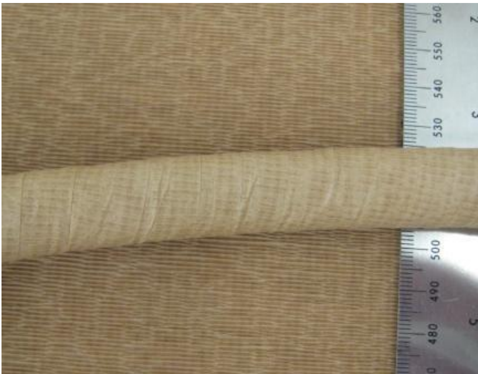
Micrex processed paper wrapped over cable
